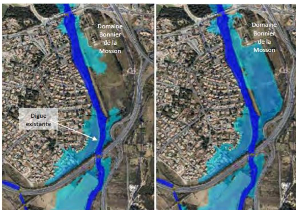
FIGURE 49 : INONDATIONS SE PRODUISANT A PARTIR D'UN DEBIT DE 200 M<sup>3</sup>/S (SOURCE EGIS EAU 2015)
